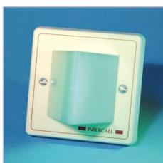
**L746 overdoor light** – these are normally positioned above doors in a corridor to indicate the status of the call point(s) within each room. The L746 can also be used to monitor several call points for end of corridor indication, or as a "follow me" light. Each unit is fitted with twin ultra-bright LED's which mimic the reassurance indicator on the call points. Also available with an integral sounder alarm (L746S).
