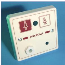
**L722 non audio call point** – specifically developed for bathrooms, toilets and other areas where the intercom facility is not required. The unit features an infra red receiver and can be activated by a TIR4 infra red trigger. The unit will accept inputs from a wide range of triggering devices including pear leads, air switches, pressure mats etc. The unit may be flush or surface-mounted using standard electrical backboxes.
